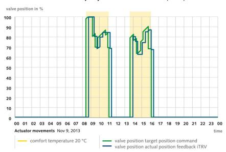
In summary, the field test shows that the energy-autonomous thermostatic radiator valve performs reliably even under the most stringent conditions—a relatively low and fluctuating inlet temperature typical for modern heating systems, a well-insulated house and the relatively warm outdoor temperatures in the transitional autumn months—and is fully equal to the battery-driven valves when it comes to convenient control.
